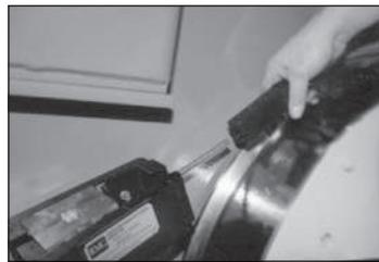
1. The head end of the wire is inserted through the Type RA pointer assembly. The gripper is attached to the wire.
