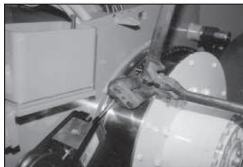
3. The reduced portion is cut with bolt cutters before removing the gripper chain and before removing the wire from the pointer assembly. Any residual fins are removed by filing.
