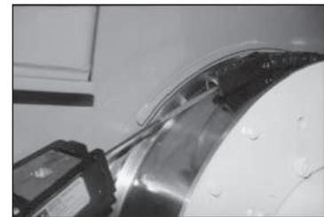
2. The machine is jogged and about 6" (150 mm) of wire is reduced to a diameter about .006" (.15 mm) to .010" (.25 mm) smaller than the finished wire diameter.
